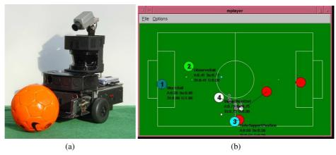
**Fig. 2.** (a) A CS-Freiburg field player, (b) a world model generated from Laser Range Finder (LRF) and camera data. The small circles represent estimates of the ball position from each robot. Large and red circles represent opponents, whereas large and enumerated circles represent teammates
