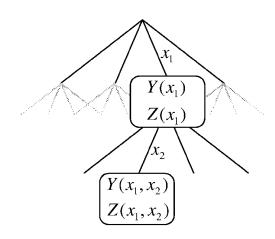
Figure 1: Querying the value of  $f^{(m)}(X)$  for  $X=(x_1,x_2)$  corresponds to traversing a path from the root to a leaf in the full tree. This path follows the edge  $x_1$  to node  $x_1$ , labeled with  $Y(x_1)=x_1$  and  $Z(x_1)=f(x_1)$ . The path then follows the edge  $x_2$  to node  $(x_1,x_2)$ , labeled with  $Y(x_1,x_2)=Z(x_1)\oplus x_2$  and  $Z(x_1,x_2)=f(Y(x_1,x_2))$ . The adversary only learns  $Z(x_1,x_2)=f^{(m)}(X)$ .
