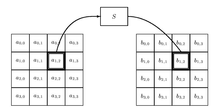
State matrix is transformed byte by byte.
