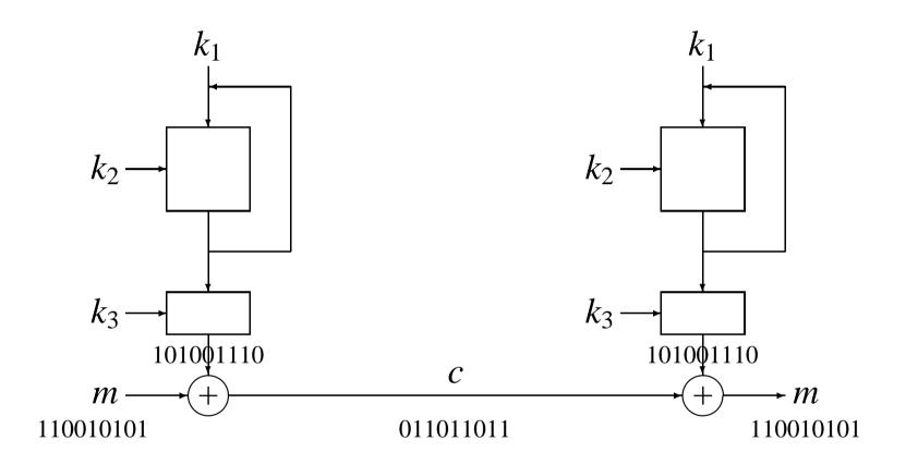
Finite state machine with output filter.
