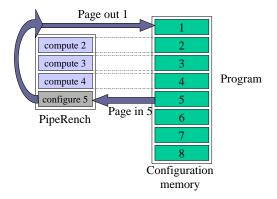
Fig. 1. Hardware virtualization in PipeRench overlaps computation with reconfiguration and provides the illusion of unlimited hardware resources.
