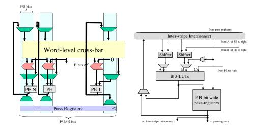
**Fig. 2.** The interconnection network between two adjacent stripes. All switching is done at the word level. All thick arrows denote *B*-bit wide connections.
