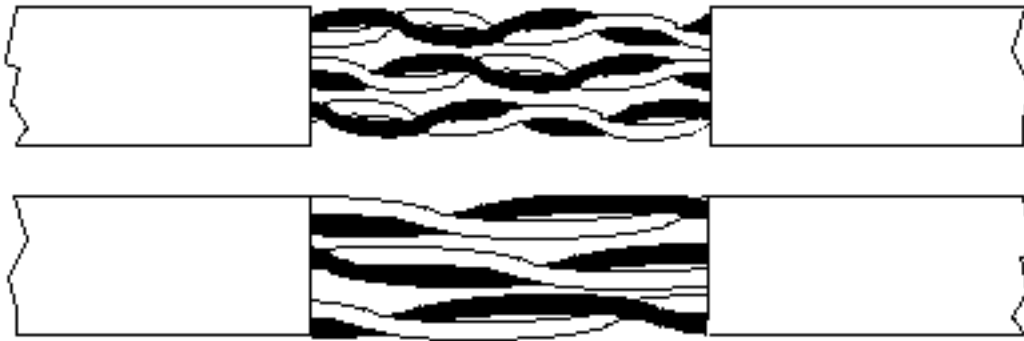
Figure 3-3. Data grade cabling has a higher number of twists per foot than voice grade cabling. The number of twists per foot within a grade declines as the number of pairs in the cable increases.
