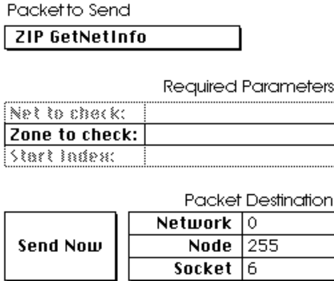
Figure 7-13. Broadcasting a GetNetInfo packet with the zone name left blank ensures that the network address range is in the same position in each GetNetInfo Reply packet.
