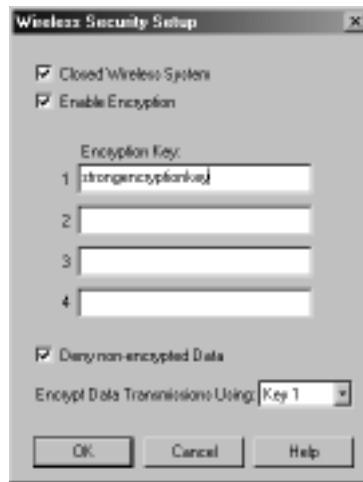
Figure 5.3 Wireless Security Setup Dialogue Box
