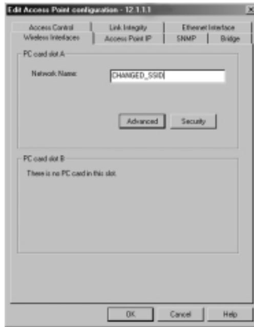
Figure 5.2 AP Configuration—Wireless Interfaces on the ORiNOCO
