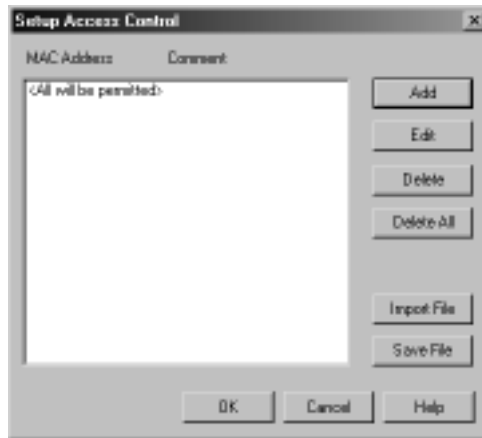
Figure 5.6 AP Setup Access Control
